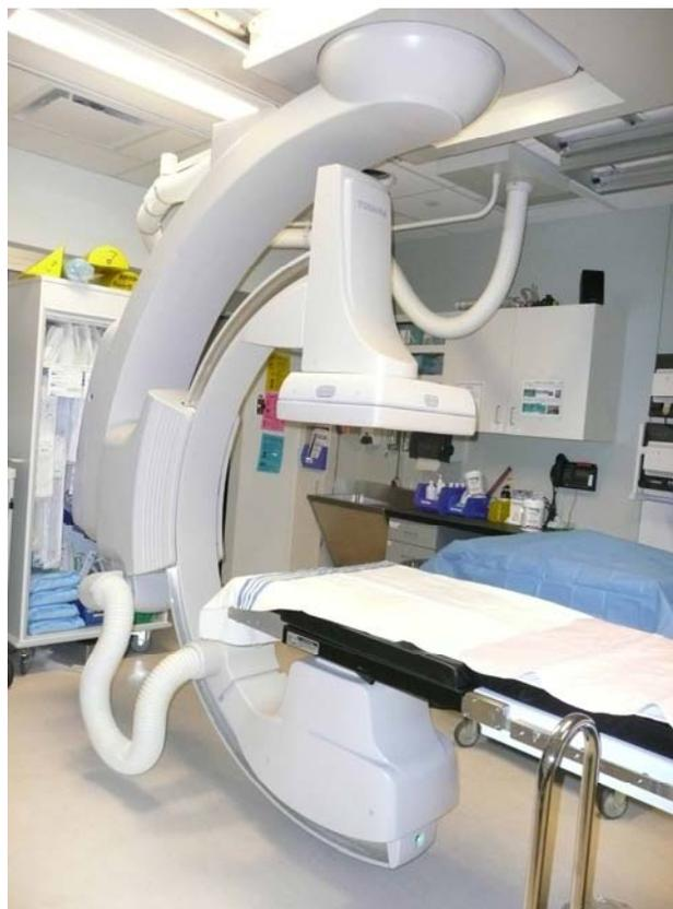
Ceiling mounted digital fluoroscopic unit with multifunctional OR table.
